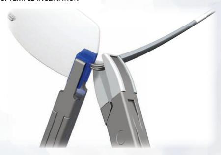
Hold side parts very frimly with the universal mounting pliers close to the area of the lens fixation. Inclinate the side parts with flat pliers. NOTE: Only bend metal parts, never plastic.
